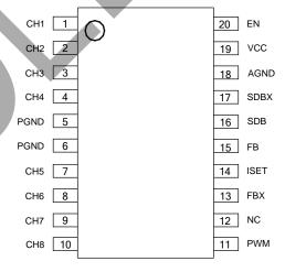
Note: AGND must be quiet and directly connected to total  $C_{\mbox{\scriptsize IN}}$
