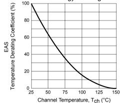
MOSFET Temperature versus Power Dissipation Curve
