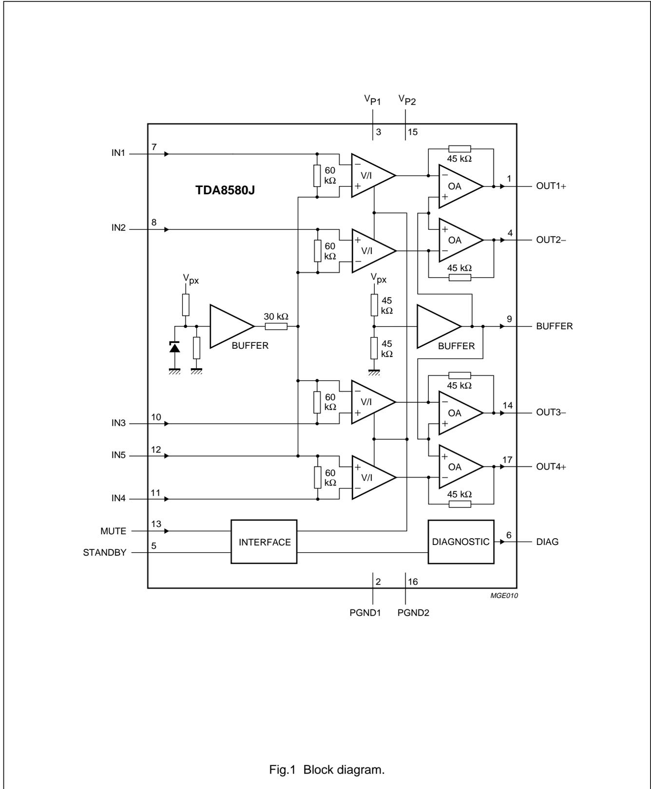
Fig.1 Block diagram.
