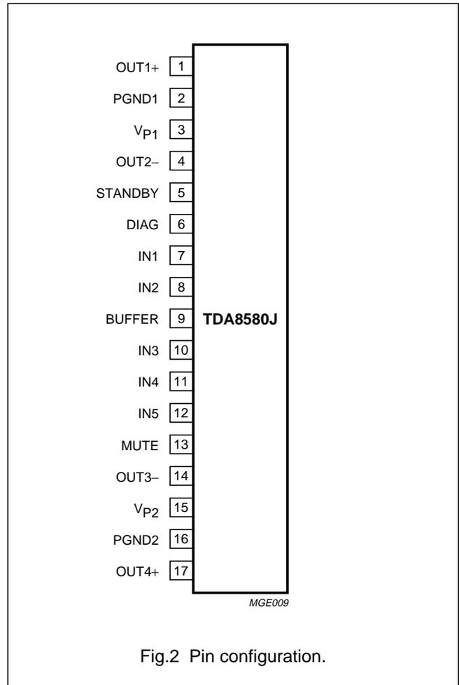
Fig.2 Pin configuration.
