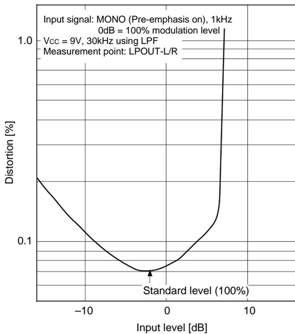
**Input level vs. Distortion characteristics 2 (Stereo)**
