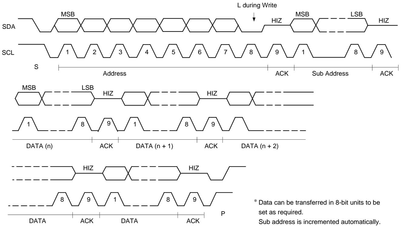
• I<sup>2</sup>C data Read (Read from the IC to I<sup>2</sup>C controller)
