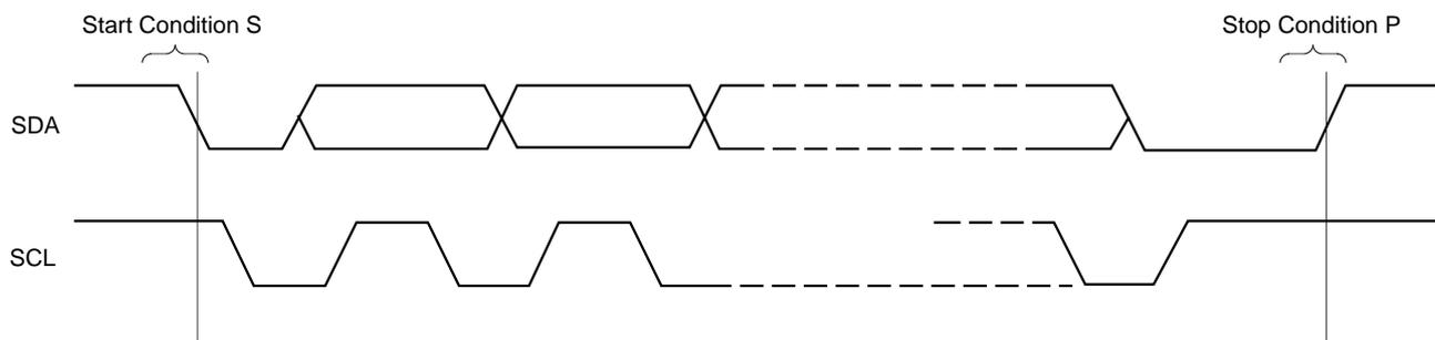
• I<sup>2</sup>C data Write (Write from I<sup>2</sup>C controller to the IC)
