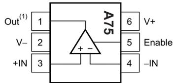
(1) Pin 1 of the 6-pin SOT-23 is determined by orienting the package marking as shown.
