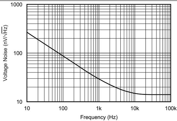
Figure 3. Input Voltage Noise Spectral Density vs Frequency
