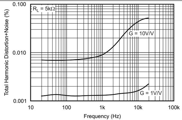
Figure 4. Total Harmonic Distortion + Noise vs Frequency
