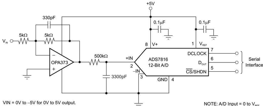
$V_{IN} = 0\text{ V to }-5\text{ V}$  for  $0\text{ V to }5\text{ V}$  output.
