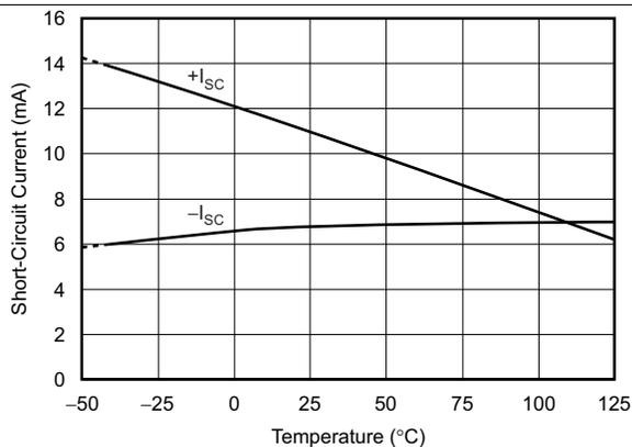
Figure 9. Short-Circuit Current vs Temperature
