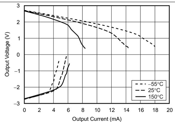
Figure 12. Output Voltage Swing vs Output Current
