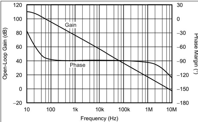
Figure 1. Open-Loop Gain and Phase vs Frequency
