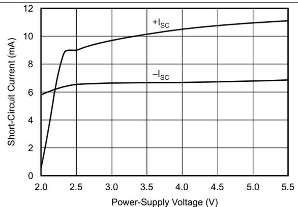
Figure 10. Continuous Short-Circuit Current vs Power-Supply Voltage
