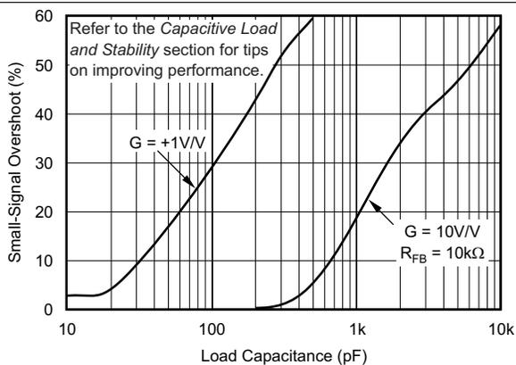
Figure 17. Small-Signal Overshoot vs Load Capacitance
