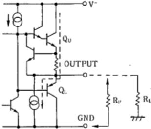
NJM2904, in its static state (No in and output condition) when design,  $Q_U$  being biased by constant current (break down beam) yet,  $Q_L$  stays OFF.
