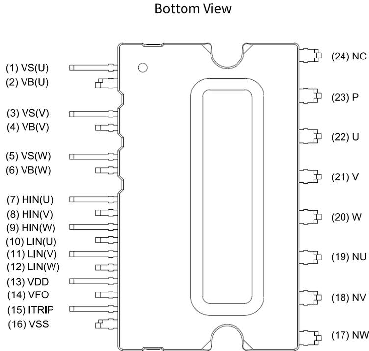
Figure 1 Pin configuration
