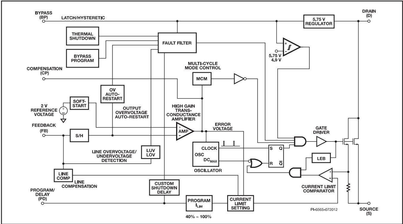
Figure 3. Block Diagram.
