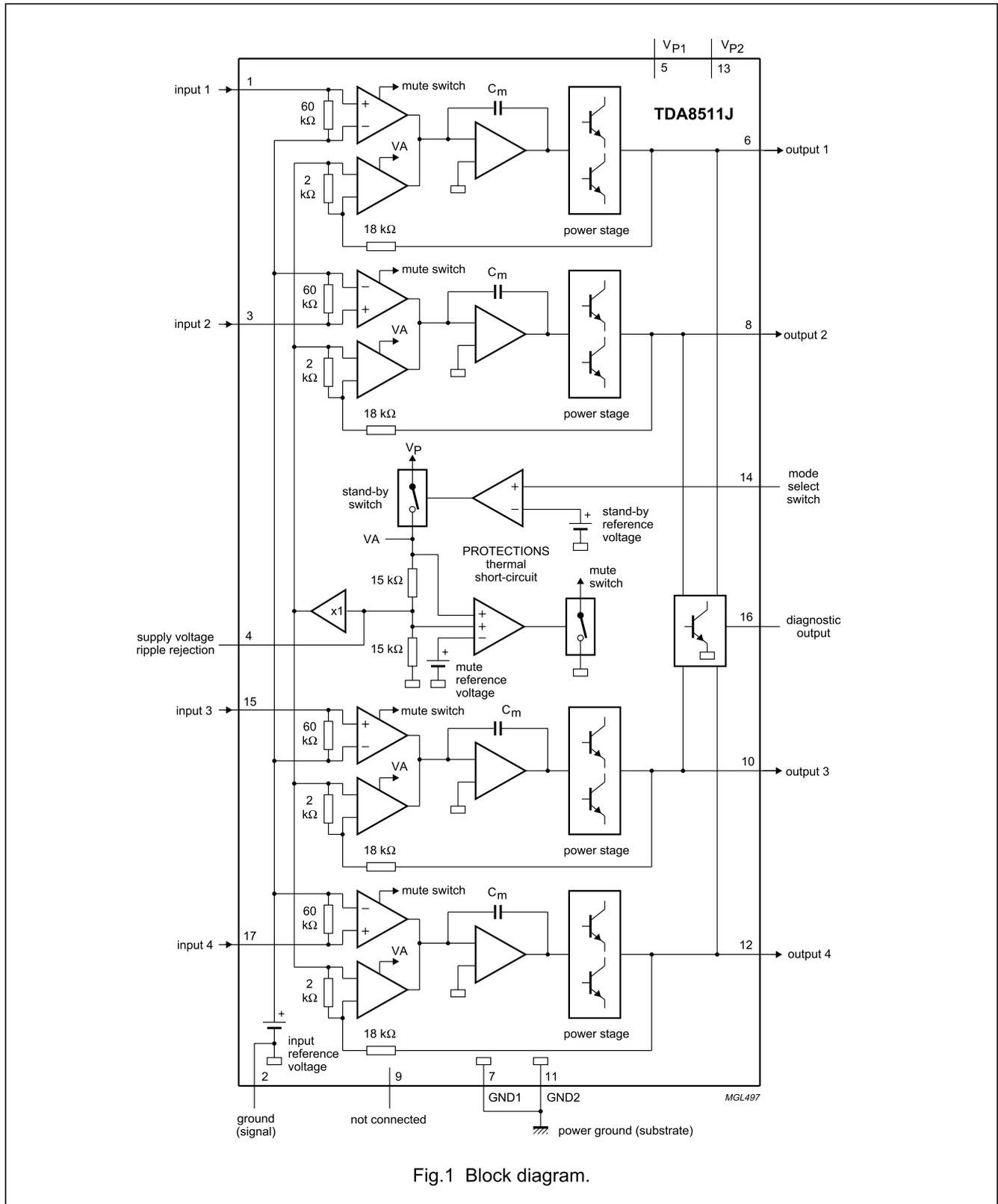
Fig.1 Block diagram.
