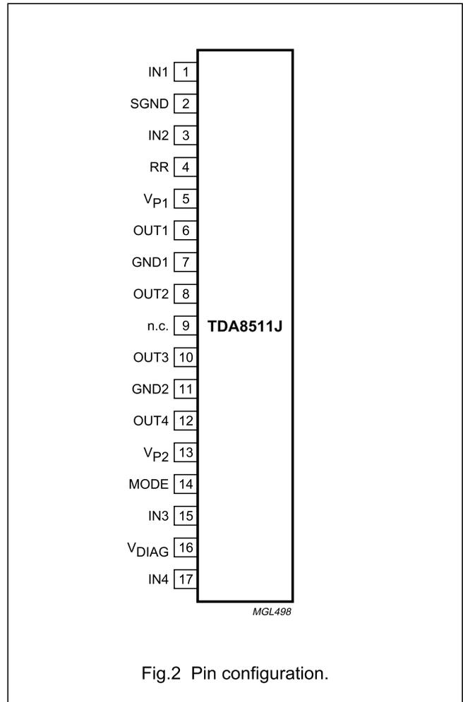
Fig.2 Pin configuration.
