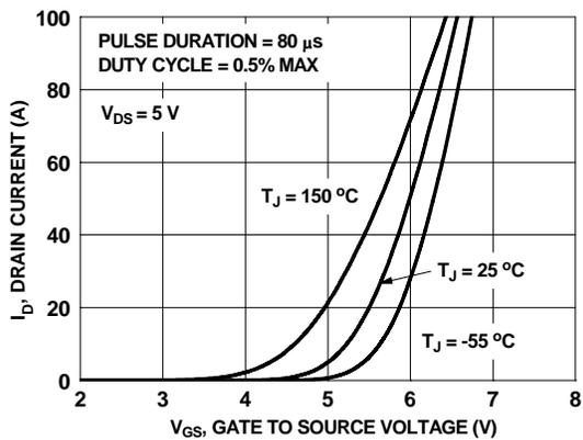
**Figure 5. Transfer Characteristics**
